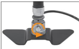
**STEP 6:** Once you are finished and **BEFORE YOU DISCONNECT THE HOSE** from whatever you are filling, slowly loosen the bleed valve to release pressure trapped in the hose.
