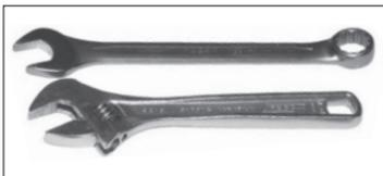
**STEP 1:** Installing a connector requires two wrenches - one for the hose and a second for the fitting. The wrench size for the hose is 14 mm. The wrench size for the fitting depends on the fitting.
