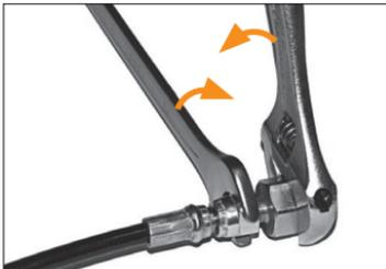
**STEP 2:** Use the wrenches to grip the hose and the fitting, then turn the hose wrench clockwise and the fitting wrench counter-clockwise until the connection is tight.
