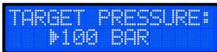
Once the desired target pressure is displayed, press the rotary control knob once to confirm the target pressure selection. After confirming the target pressure selection, the start display at the end of the main menu will appear.
