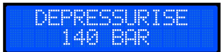
When the compressor detects that the pressure is low (roughly below 70 BAR / 1015PSI) the display will return to the main menu.
