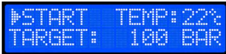
With the start display visible, press the rotary control knob once to start the compressor. After starting the compressor, the running display will appear.
