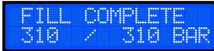
**DO NOT** disconnect the vessel until the compressor has been fully depressurised.
