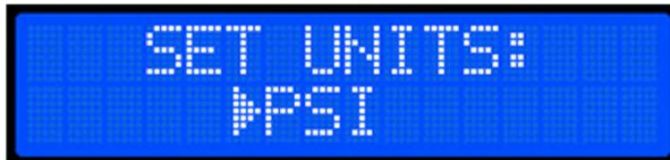
Rotate the rotary control knob in either direction to cycle between the selectable units. Once the desired unit is visible, press the rotary control knob once to save the selection. The compressor will retain the selected pressure unit, even after being powered off.
