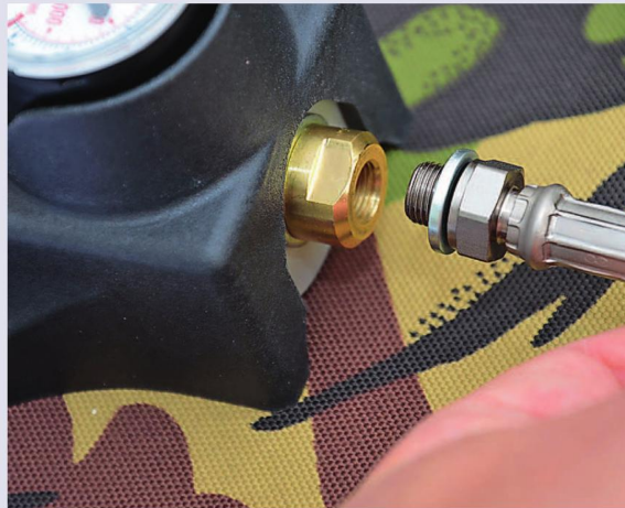
5. Attach the air line
