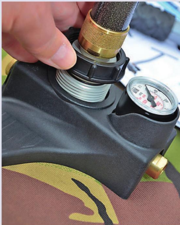
4. Lock it in place with the collar
