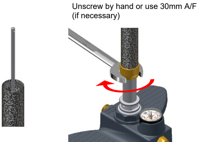
4. Unscrew outer body tube end cap and remove body tube
