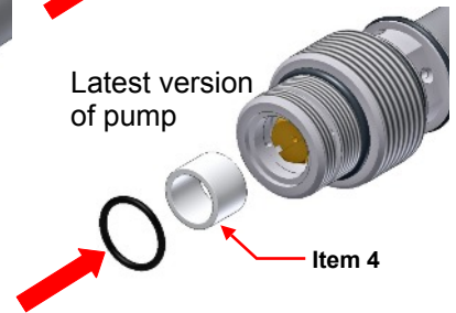
B5. Fit new micron filter Item 4 and re-assemble
